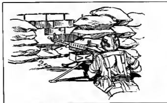
Figure 5-38. Use of a loophole with a machine gun.
